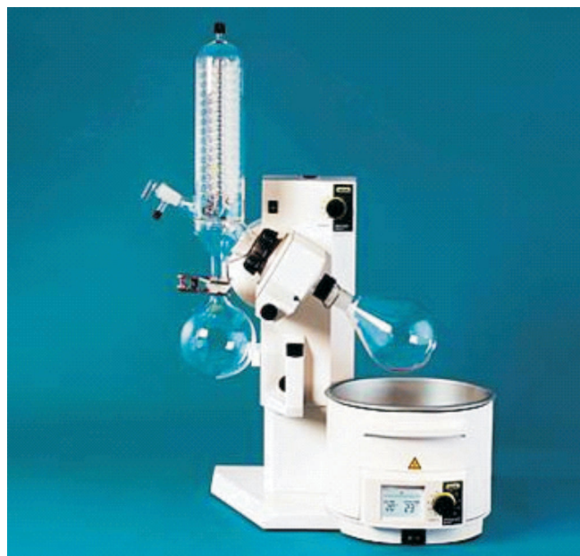
Fig-2: Rotary flash evaporator
